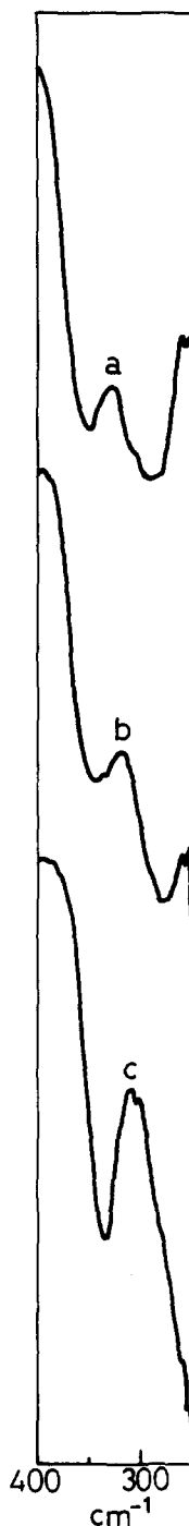
FIG. 3. Cation–oxygen stretching bands for: (a) x = 2 , (b) x = 5 , (c) x = 8 .
